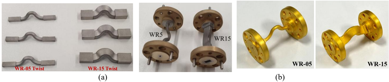
Fig. 1. Photographs of the mm-wave twist waveguides: (a) As-printed waveguide twist sections; (b) Assembled with the flanges and after AFM polishing and after gold plating.
